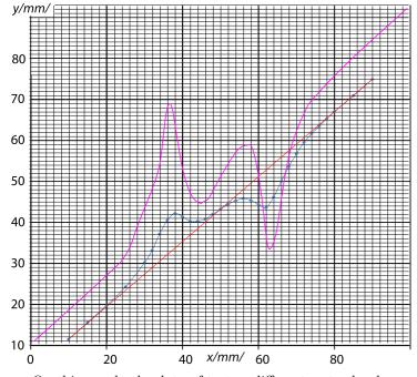
On this graph, the data of to two different water levels are depicted; blue curve corresponds to a water depth of  $ca \ 2 \ mm$  (data given in the table above); the violet one — to 1 mm.
