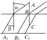
$$\frac{v_1}{v_2} = \frac{A_1 B_1}{B_1 C_1} = \frac{AB t g \alpha}{BC t g \beta} = \frac{t g \alpha}{t g \beta}.$$
