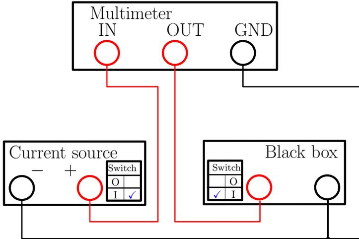
i. (1 pt) During charging of the capacitor from  $V = 0$  to  $V = V_{\max}$  we note that the output of the current source is constant ( $I_0 = 6.0$  mA) close to the precision of the multimeter.
